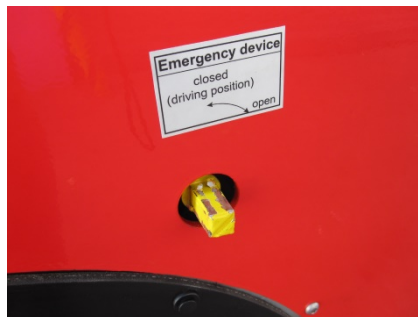
Emergency device „opened“ (vehicle can be lowered)
